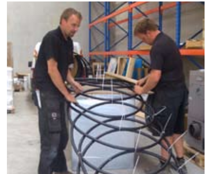
Manufacturing a 'slinky' ground loop pipe
