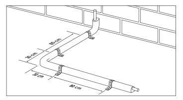
If MULTITUBO multi-layer pipes are installed on the floor or in the supporting floor, a fastening distance of 80 cm has to be observed. The distance between each bend and the fixing device before and after it must be 30 cm.
