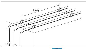
If MULTITUBO multi-layer pipes are openly installed on the ceiling, additional pipe supports are not necessary. The following chart shows the maximal fastening distances between the individual pipe clamps for the different pipe dimensions.
