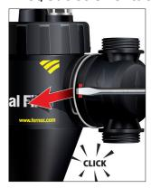
1. Using a flat end screwdriver in the recess shown, gently lever the locking clip into the 'unlock' position.
