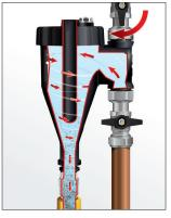
3. Open outlet and drain valves
