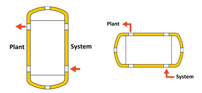
Where it is not possible to connect the tank on opposite sides it is acceptable to make the system and plan connections both on the same side of the tank.
