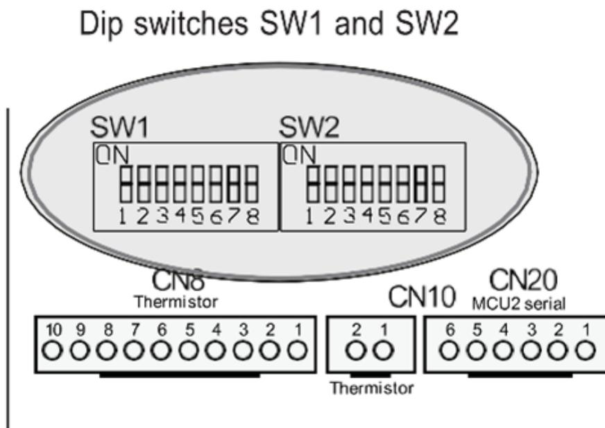
The manual includes tables that show the full functions of each dip switch, although most of these do not need to be changed by the installer.
