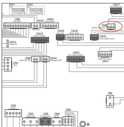
Isolate the power supply and remove black plastic cover from the PCB. Connect field wiring to the cable tail (two white wires) connected to the boilers CN9 PCB connector. Any field wiring must be a minimum of 0.5mm<sup>2</sup> shielded cable and not exceed a total length of 50m. This connection to CN9 is low voltage only and **must not have 230VAC applied to it.**
