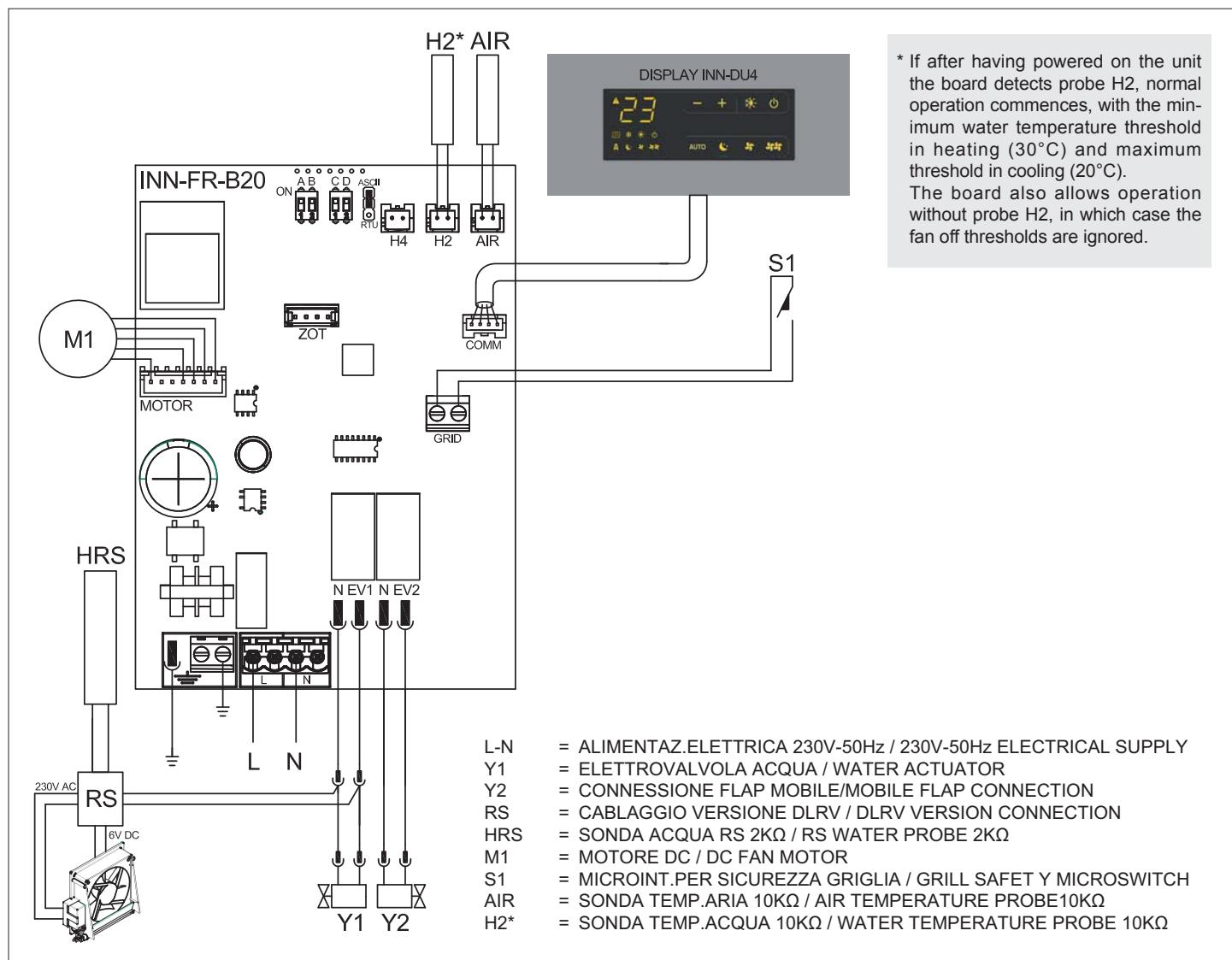
\* If after having powered on the unit the board detects probe H2, normal operation commences, with the minimum water temperature threshold in heating (30°C) and maximum threshold in cooling (20°C).
