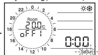
Note: Press the Return button to return to the previous item. Press the Timer for Heating/Cooling button for 3 seconds again to return to normal operation, or simply do nothing for approximately 2 minutes.
