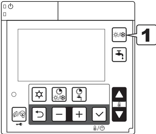
**1** Press the Mode (Heating/Cooling) button to select Heating/Cooling mode.
