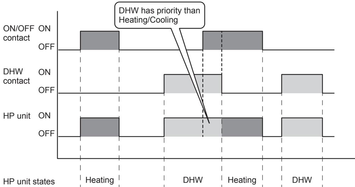
Note2: In case the ON/OFF remote contact is enabled and Heating/Cooling remote contact is disabled (by Remote controller), if the ON/OFF remote contact=ON and Heating or Cooling is in operation, and if the Mode button of Remote controller is used to select OFF among Heating→Cooling→OFF, the ON/OFF remote contact=ON condition will be top priority than the Mode button of Remote controller.
