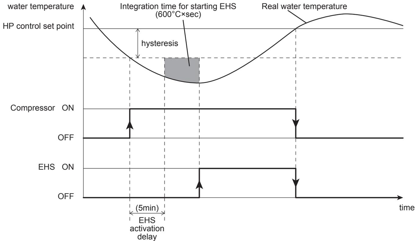
The “HP control set point” is equal to the value set for Fixed set point control, or by the value determined by the Climatic curve.
