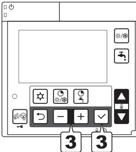
**3** When the DHW Comfort icon displays and DHW Comfort set point (Default: 50°C) blinks, change the DHW Comfort set point using the - or + button, and press Set button to save the setting.
