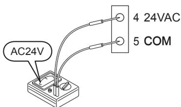
[Fig. 11] Voltage of 3way mixing valve (control)
