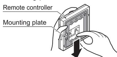
2. Fix the mounting plate to the wall.
