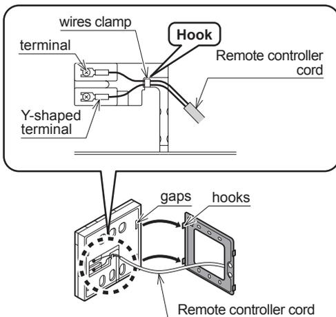
**When the wiring is exposed**
