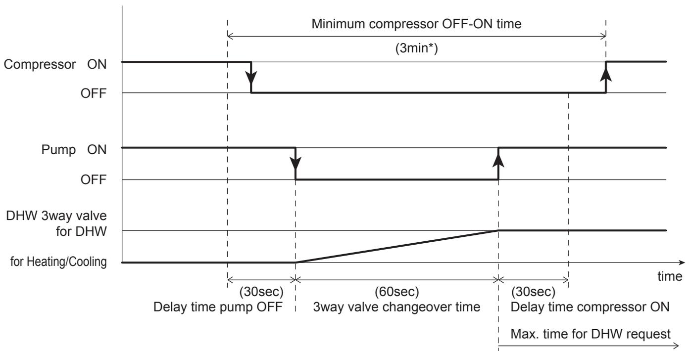
\*Minimum compressor OFF-ON time (3min) is a fixed value. The interval time is necessary for refrigerant cycle safety, it cannot be changed.
