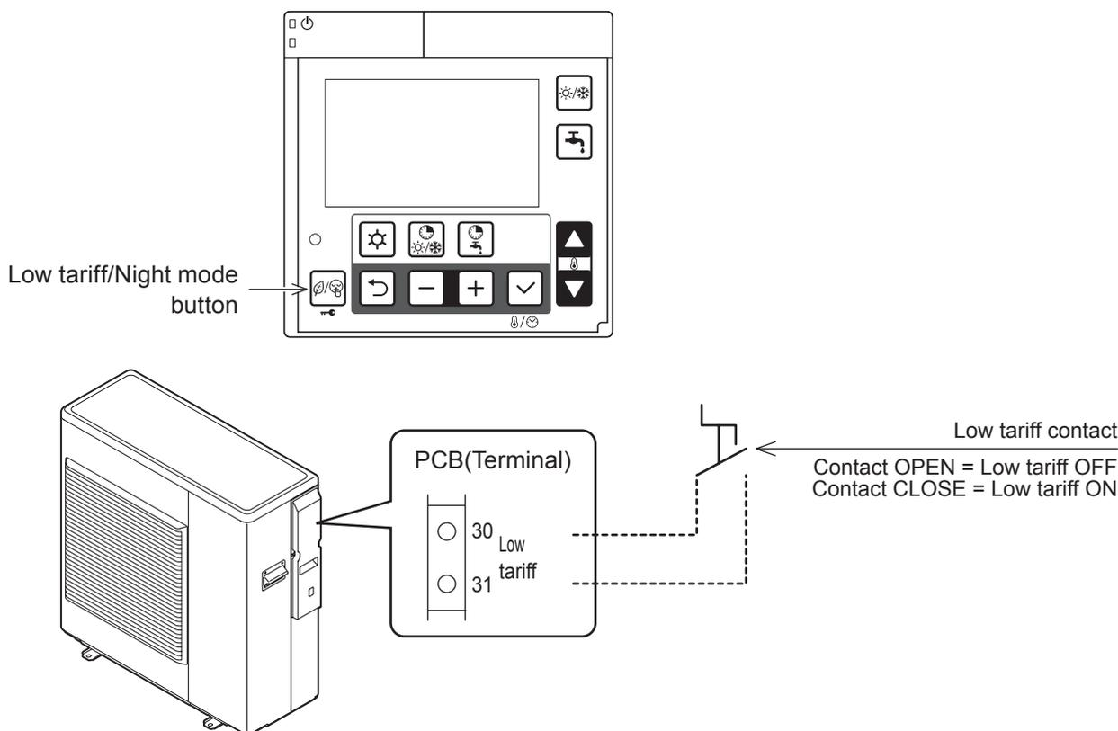
Note1: Par5128 (Night mode) and Par5130 (Low tariff) are automatically synchronized to same value. If Par5128 is changed to 1 (enable), then Par5130 will be also changed to 1 (enable).
