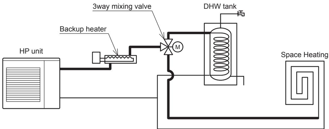
A parameter defines if the Backup heater can be enabled or disabled, and the “Type of function”:
