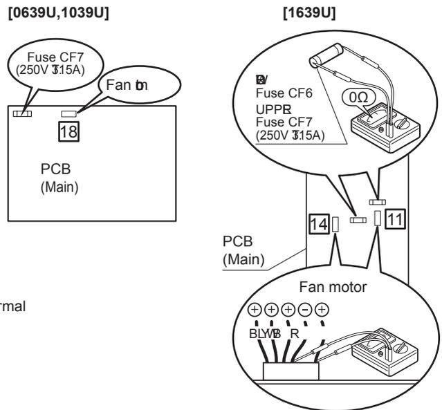
[Fig. 3] Continuity of current Fuse on the PCB (Main)
