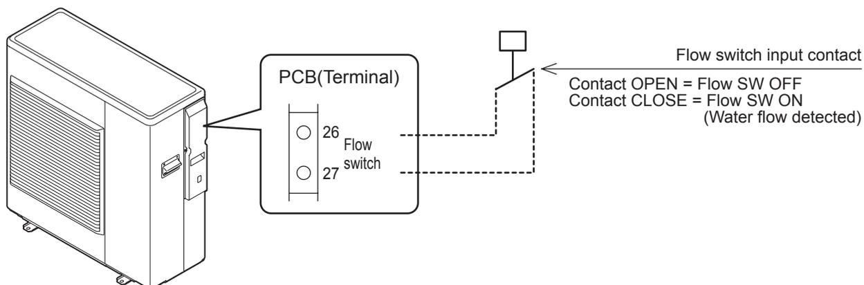
At Start-up, the compressor will not be turned ON unless the flow switch is CLOSED (water flow detected).
