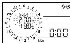
Then the Economy icon displays and set point temperature (Default: 18.0°C) blinks. And change the Economy set point temperature by using the - or + button, and press the Set button to save the setting.
