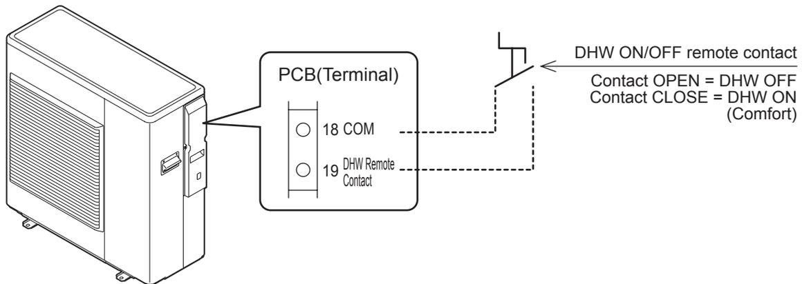
Note1: In order to use DHW function, it is necessary to set Par3101=1or2, and Par5107=1.
