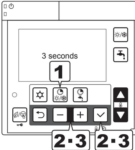
**1** Press the Timer for Heating/Cooling button for 3 seconds to set the time bands for Heating/Cooling.
