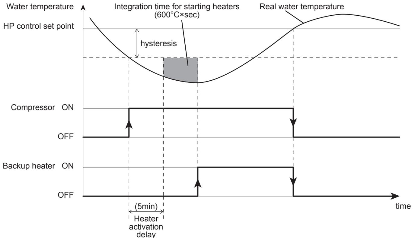
The “HP unit control set point” is equal to the value set for Fixed set point control, or by the value determined by the Climatic curve.
