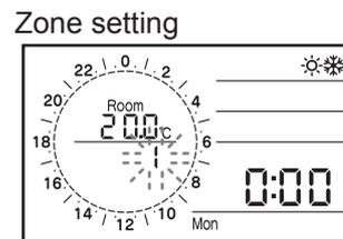
**3** When the Zone has been saved, the day of week (Default: Mon) blinks. Specify the day of the week using the - or + button and then press the Set button to save the setting. The time bands can be programmed by selecting the days in present group or for each individual day.
