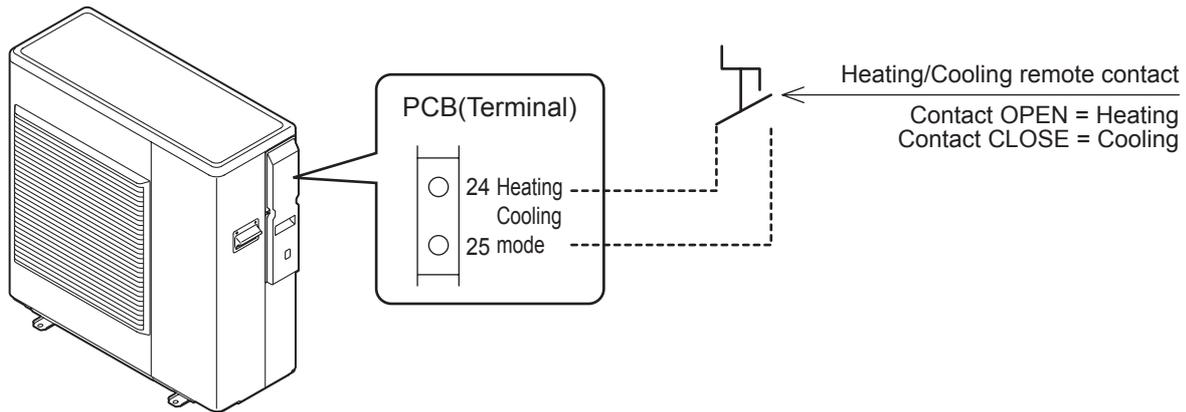
Note: Heating/Cooling remote contact will be used when the operation of HP unit is turned ON by ON/OFF remote contact. It is not available if ON/OFF remote contact is OFF, and set Par5120=0.
