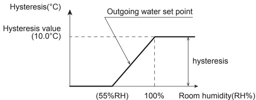
Note: If the HP unit is connected directly to the system, without Buffer tank, the maximum Room humidity compensation has effect on the Outgoing water temperature from the HP unit. If the HP unit is connected to the Buffer tank and the low temperature Zone with a 3way mixing valve is enabled, the maximum Room humidity compensation has effect on the Outgoing water temperature from mixing valve.
