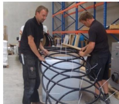
*Manufacturing a 'slinky' ground loop pipe*
