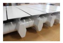
When the sections are connected, tighten the joints so the gaskets are firmly compressed. A tightening torque of 100 lbf-ft must be applied.
