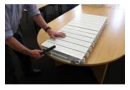
One turn at a time, rotate the nipple using the nipple key. This will pull the two sections together. After one turn, repeat with the other nipple. Continue to alternate between the nipples, one turn at a time, until the two sections are pulled together. It is important to keep the sections parallel to one another.
