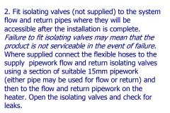
Where hoses are not supplied (SS3) connect the heater to the isolating valves using pipe work suitable for LPHW (Low Pressure Hot water systems) which will allow access to the product once installed.
