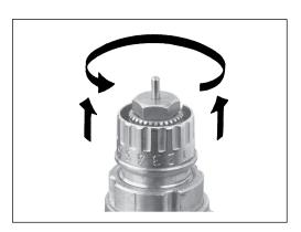
Danfoss pre-settable valve bodies incorporate easy setting adjustment rings with clearly engraved setting markers scaled from 1 - 7 and N. Setting values can be set quickly and precisely, without the need for tools, as follows:
