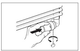
The self-sealing gland is mounting in radiator inlet and outlet using a 17 mm hexagonal key.
