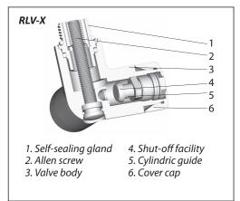
The valve assembly features valve body and a self-sealing gland pre-mounted with 2 O-rings - one for sealing against the radiator and one for sealing in the valve housing.
